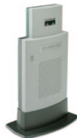
Cisco Aironet 1100 Series Built-in .11b, future .11g
